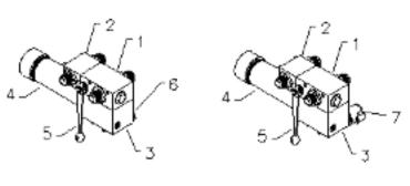
Manual Electric Figure 3.7: The On / Off valve
