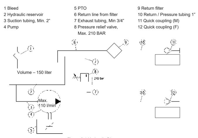
Figure 2.1 Hydraulic Diagram
