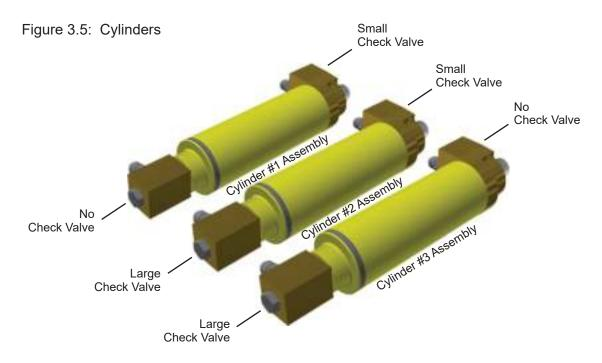
The above figure shows the difference between the cylinder compilation.
