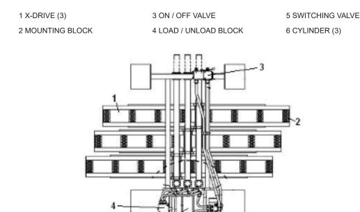
Figure 3.1: KEITH® WALKING FLOOR® Workhorse drive-unit
